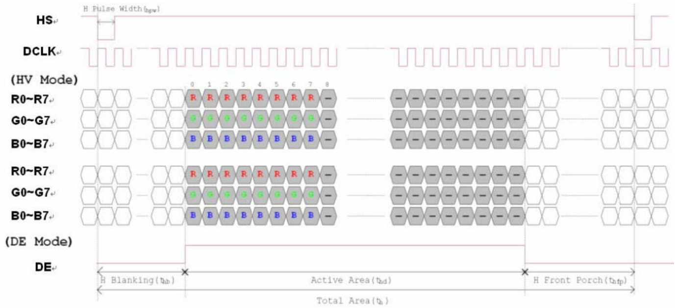
Figure 3.1 Horizontal input timing diagram
